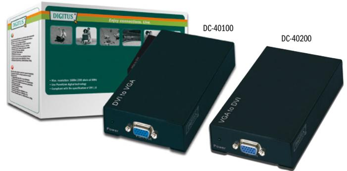
This conversion box converts a digital signal from a DVI video source to an analog signal. So it is for example possible to use an old analog monitor with a new DVI graphic card.
